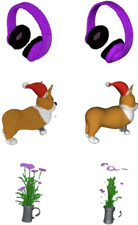
Figure 7. Examples of point clouds (left) and corresponding extracted meshes (right). We find that our method often produces smooth meshes and removes outliers (middle row), but can sometimes miss thin/sparse parts of objects (bottom row).
